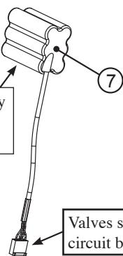
Valves shipped with battery not connected to circuit board. Connect this end to circuit board.
