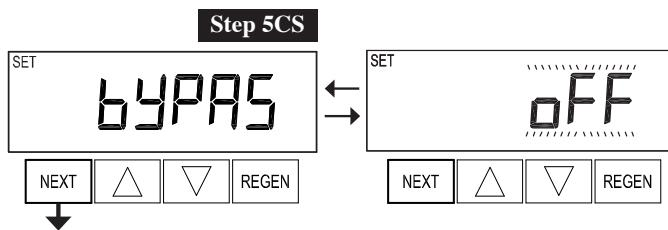
**Step 5CS** – This display will not appear if 1.0T was selected in Step 2CS. Allows selection of one of the following using **▲** or **▼**:
