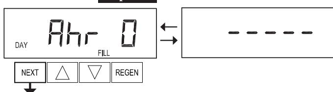
**Step 4BD** – Battery Pack Charge History. Displays the measure mAh charge of the battery pack over the past 63 days. **REGEN** in the second display indicates that a regeneration occurred on that day. Press **NEXT** to exit Battery Diagnostics. Press **REGEN** to return to previous step.
