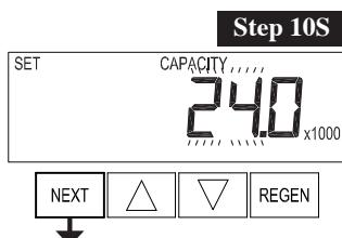
**Step 10S** – Set System Capacity using **▲** or **▼**. The System Capacity setting should be based on the volume of resin and LBS of salt fill set in Step 9S. Press NEXT to go to Step 11S. Press REGEN to return to previous step.
