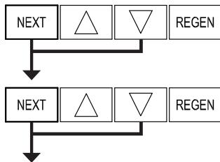
**Step 1CS** – Press NEXT and ▲ simultaneously for 5 seconds and release. Press NEXT and ▼ simultaneously for 5 seconds and release. If the screen in Step 2CS does not appear, the lock on the valve is activated. To unlock, press ▼, NEXT, ▲ and REGEN in sequence, then press NEXT and ▼ simultaneously for 5 seconds and release. Press NEXT and ▼ simultaneously for 5 seconds and release.
