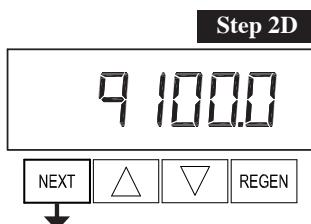
**Step 2D** – Software Version. Press **NEXT** to go to Step 3D. Press **REGEN** to exit Diagnostics.
