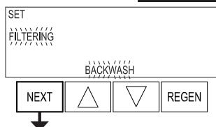
**Step 2F** - Choose FILTERING BACKWASH or FILTERING REGEN (see table) using ▲ or ▼. Press NEXT to go to Step 3F. Press REGEN to exit OEM Filter System Setup.
