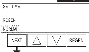
**Step 6F** - Set Regeneration Time Options using ▲ or ▼. NOTE: This step will not appear if Step 5F is set to oFF.
