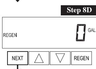
**Step 8D** – Volume, since last regeneration: This display shows the volume of water that has been treated since the last regeneration. This display will equal zero when a water meter is not installed. Press **NEXT** to go to Step 9D. Press **REGEN** to return to previous step.
