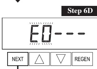
**Step 6D** – Error Log: This display shows a history of the last 10 errors generated by the control during operation. Press **▲** or **▼** to view each recorded error.
