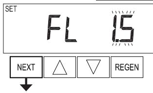
**Step 3CS** – If 1.5 or 2.0 is selected in Step 2CS, an additional screen will appear. It is used to select which size flow meter is to be used with the valve, 1.0r, 1.5, 2.0 or 3.0. Variable meter pulses of 0.1-150.0 PPG can also be selected. Press NEXT to go to Step 4CS. Press REGEN to return to the previous step.
