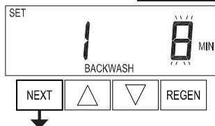
**Step 3F** - Select the time for the first cycle using ▲ or ▼.
