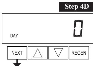
**Step 4D** – Days, total since start-up: This display shows the total days since startup. Press the **NEXT** button to go to Step 5D. Press **REGEN** to return to previous step.
