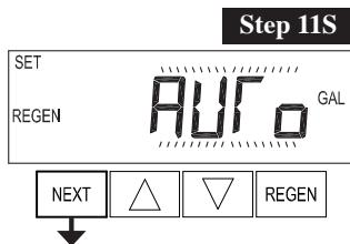
**Step 11S** – Set Volume Capacity using **▲** or **▼**. If value is set to:
