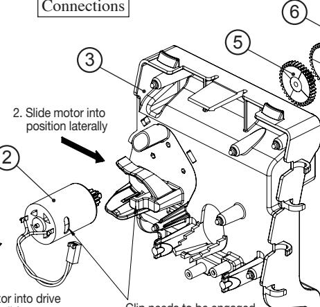
2. Slide motor into position laterally
