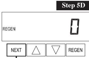
**Step 5D** – Regenerations, total number since start-up: This display shows the total number of regenerations that have occurred since startup. Press the **NEXT** button to go to Step 6D. Press **REGEN** to return to previous step.
