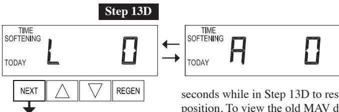
**Step 13D** – MAV Drive History in the direction of extended piston rod position. Display will only be shown if 1.0Γ is selected in Step 2CS, or OFF is not selected in Step 4CS. Up to a four digit number will appear after the “L” which stands for latest and “A” which stands for average. Drive time is measured in 1/100 of a second; i.e., a 17.15 second move is displayed as “1715”. Press and hold ▲ and ▼ for 3
