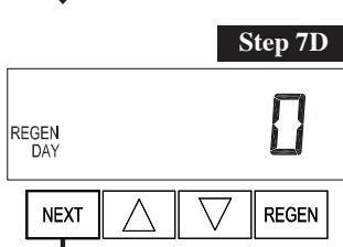
**Step 7D** – Days, since last regeneration: This display shows the days since the last regeneration occurred. Press **NEXT** to go to Step 8D. Press **REGEN** to return to previous step.
