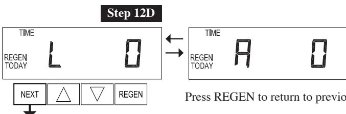
**Step 12D** – MAV Drive History in the direction of retracted piston rod position. Display will only be shown if 1.0Γ is selected in Step 2CS, or OFF is not selected in Step 5CS. Up to a four digit number will appear after the “L” which stands for latest and “A” which stands for average. Drive time is measured in 1/100 of a second; i.e., a 17.10 second move is displayed as “1710”. Press NEXT at any time to go to Step 13D.
