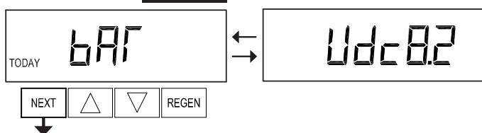
**Step 2BD** – Battery Pack Status – Pack Voltage. Displays the daily measured voltage of the battery pack under load. Press and hold **▲** and **▼** to initiate an immediate test of the battery pack. Press **NEXT** to go to Step 3BD. Press **REGEN** to exit Battery Diagnostics.
