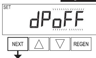
**Step 4CS** – Selecting the use of an outside signal to initiate a regeneration: Selection only matters if a connection is made to the two pin connector labeled DP SWITCH located on the printed circuit board. Following is an explanation of the options:
