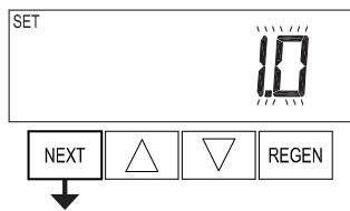
**Step 2CS** – Use ▲ or ▼ to select 1.0 for 1" valve, 1.25 for 1.25" valve, 1.5 for 1.5" valve, 2.0 for 2" valve or 1.0T for twin valve. Press NEXT to go to Step 3CS. Press REGEN to exit Configuration Settings.
