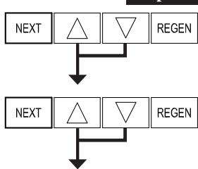
**Step 1BD** - Press **▲** and **▼** simultaneously for 5 seconds and release. Press **▲** and **▼** simultaneously for 5 seconds and release. If screen in Step 2BD does not appear the lock on the valve is activated. To unlock press **▼**, **NEXT**, **▲**, **REGEN** in sequence, then press **▲** and **▼** simultaneously for 5 seconds (twice) and release.
