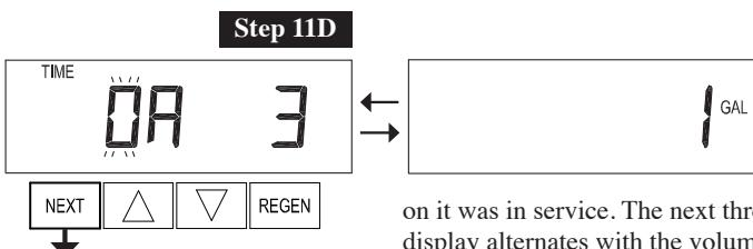
**Step 11D** – Twin Tank Valve transfer history: only displays when 1.0Γ was selected in Step 2CS. Use ▲ or ▼ to scroll through the last 10 tank transfers. The first position in the display ranges from 0 to 9 with the lowest number being the most recent transfer. The second position in the display will be either “A” or “b”. If “A” then the tank with the valve on it was in service, if “b” the tank with the in/out head
