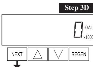
**Step 3D** – Volume, total used since start-up: This display shows the total gallons treated since startup. This display will equal zero if a water meter is not installed. Press the **NEXT** button to go to Step 4D. Press **REGEN** to return to previous step.
