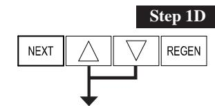
**Step 1D** - Press **▲** and **▼** simultaneously for 5 seconds and release. If screen in Step 2D does not appear the lock on the valve is activated. To unlock press **▼**, **NEXT**, **▲**, **REGEN** in sequence, then press **▲** and **▼** simultaneously for 5 seconds and release.
