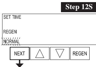
**Step 12S** – Set Regeneration Time Options using **▲** or **▼**. NOTE: This step will not appear if Step 11S is set to oFF or Step 5CS is set to “SYS”.
