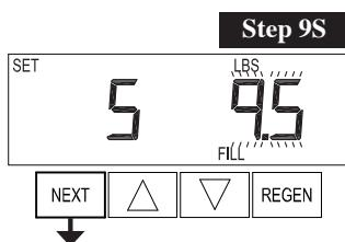
**Step 9S** – Select the pounds for the fifth cycle using **▲** or **▼**. For valve types 1.5 and 2.0, “oFF” is also available.
