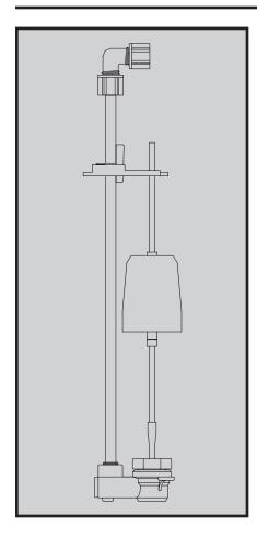
Our popular 434 Brine Valve is available in three models; Standard, Control Flow and High Flow to allow you to choose the best model for your application. The 434 Brine Valve can be used on residential and light commercial applications refilling up to one gallon per minute. The 434 is a non-air check brine valve. The Standard model is designed for use on systems utilizing non-timed refill. The Control and High Flow models are designed for timed refill systems.
