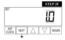
**Step 3F**—Valve Type: Select valve type using  $\nabla$  or  $\triangle$ . Available selections are 1.0 or 1.25. Press NEXT to go to Step 4F. Press REGEN to return to previous step.
