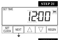
Step 2U—Current Time (hour): Set the hour of the day using ▼ or ▲. a.m./p.m. toggles after 12. Press NEXT to go to Step 3U. Press REGEN to exit Set Time of Day.
