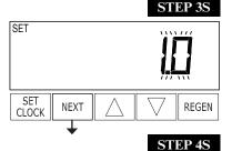
**Step 3S**—Valve Type: Select valve type using **▼** or **△**. Available selections are *1.0* or *1.25*. Press NEXT to go to Step 4S. Press REGEN to return to previous step.
